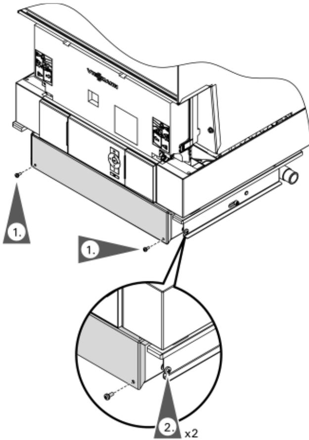
**Accessing the control unit connections**
