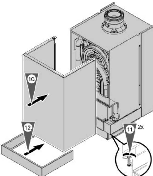
10. Set front enclosure panel on the guide rails and push in place.
