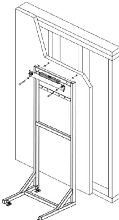
The Vitodens 200-W, model B2HA does not come with a mounting template. The wall location for the frame, mounting bracket and all vents must be field calculated.
