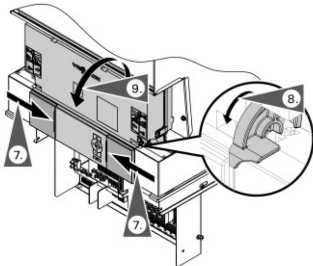
7. Slide both sides of the programming unit cover closed.
