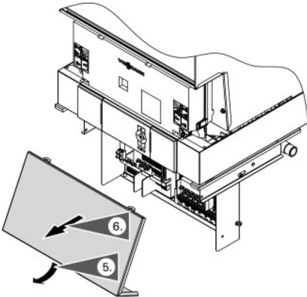
5. Tilt the bottom of the external accessory connection box cover forward.
