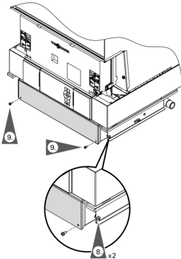
8. Tighten the external accessory connection box retaining screw.
