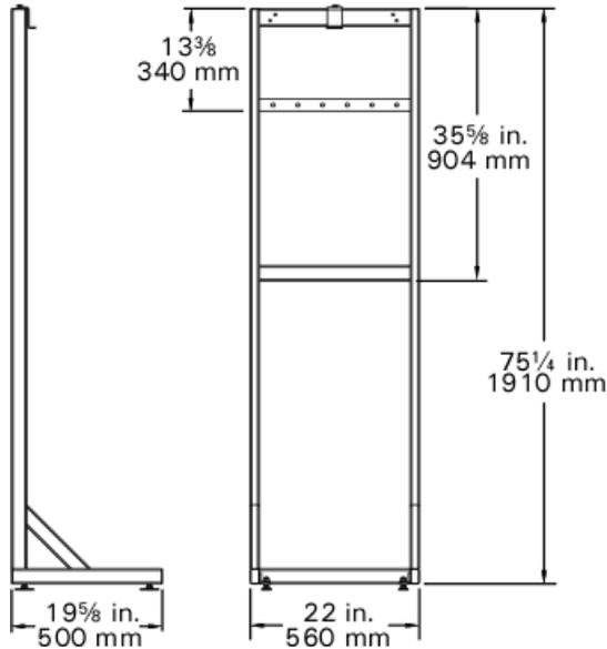
The boiler stand is used for free-standing installation of a single boiler within the mechanical room.
