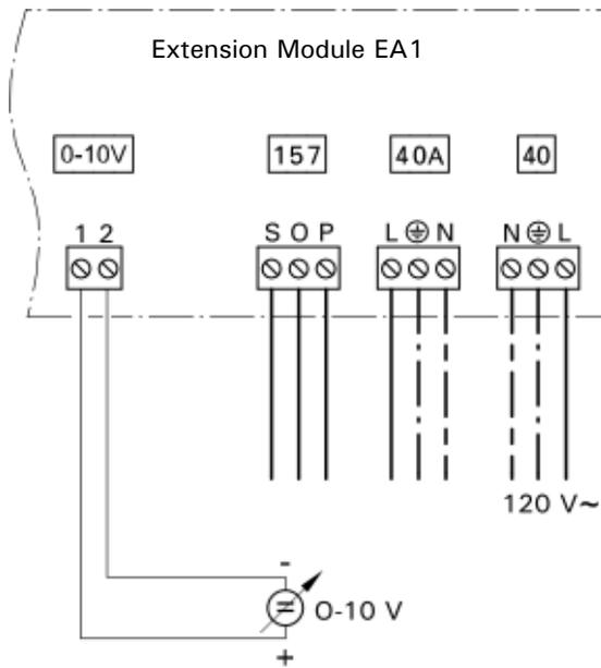
1. Connect the external 0-10V signal to plug 0-10V located in the extension module EA1.
