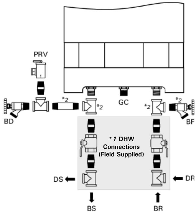
Use an approved pipe sealant or teflon tape when connecting the following installation fittings.
