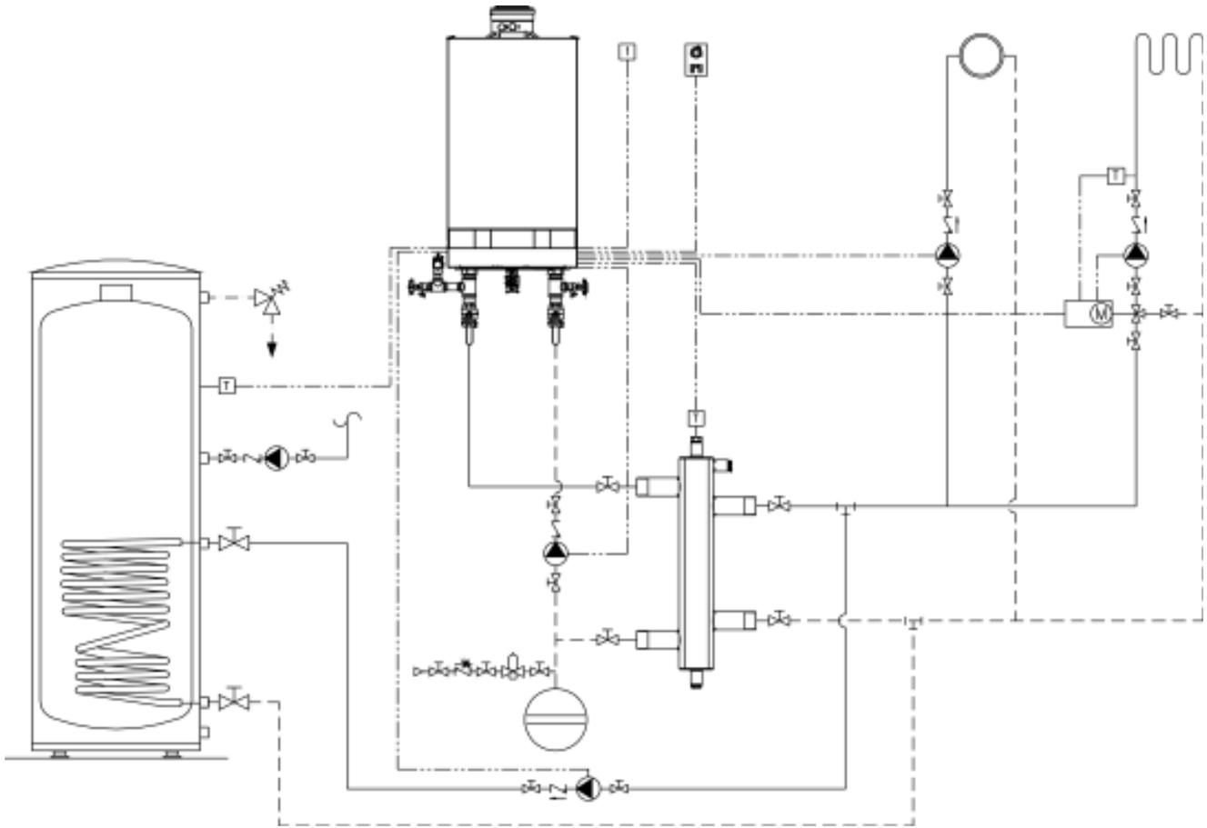
**\*Note:** When using a low loss header in the system, the DHW connections can be made downstream of the low loss header. See Vitodens 200-W B2HA Service Instructions for applicable system coding information (see coding level 2):
