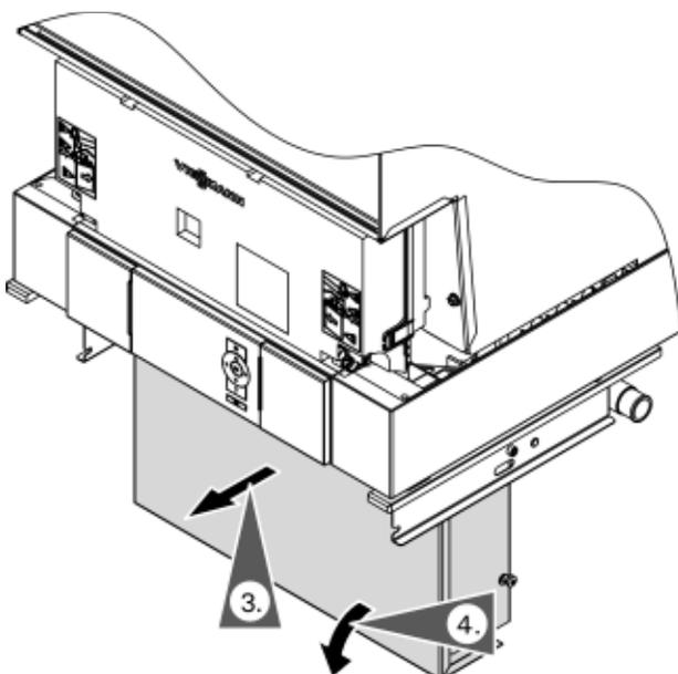
3. Pull the external accessory connection box forward until the retaining screws are clear of the guides.
