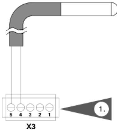
1. Connect the low-loss header sensor (if used) to terminals X3.4/X3.5 on the boiler control board.
