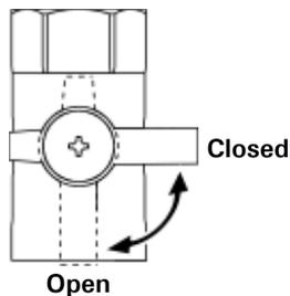
**Gas shut-off valve connection**
