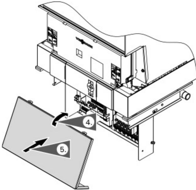
4. Tilt the top of the external accessory connection box cover forward.
