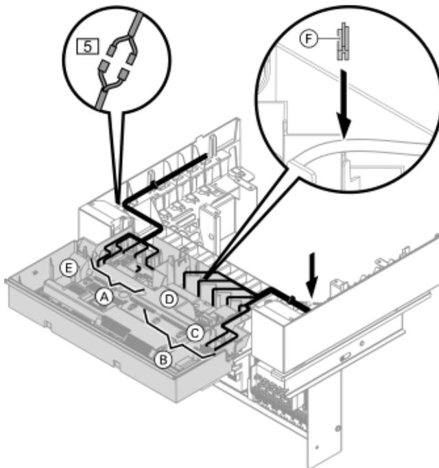
**Routing the connecting cables**
