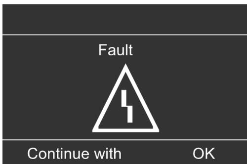
If any faults have occurred in your heating system, the symbol flashes in the display, and “Fault” appears. The red fault indicator also flashes (see chapter “Starting the heating system”).
