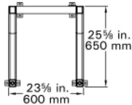
The boiler stand is used for free-standing installation of a single boiler within the mechanical room.
