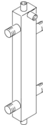
When used in conjunction with the Vitodens 200-W boiler, the low-loss header acts as hydraulic break, decoupling boiler and system circuits from each other. It is recommended to use the low-loss header in applications in which the total system flow rate exceeds the maximum (or minimum) boiler flow rate. For maximum boiler flow rates, see page 9 of this manual.
