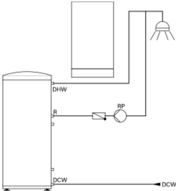
DHW recirculation lines increase the level of comfort and convenience of the domestic hot water supply and reduce water consumption.
