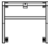
The boiler stand is used for free-standing installation of a single boiler within the mechanical room.
