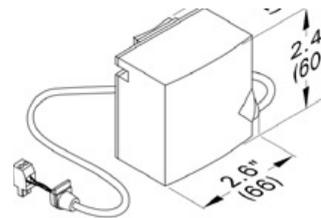
Installed with a strapping band.
