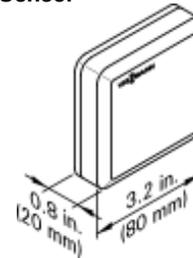
Separate room temperature sensor as supplement to the Vitotrol 200A and 300A; to be used if the Vitotrol 200A or 300A cannot be installed inside the main living room or in a suitable position where the unit can capture and adjust the temperature.
