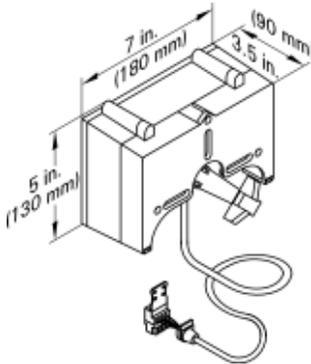
The mixing valve actuator is mounted directly on the Viessmann ¾ to 2½" mixing valve. The mixing valve actuator is a motor-driven control unit. The rotational direction is reversible. The mixing valve actuator comes with a plug-in connector for a heating circuit pump, supply temperature sensor (strap-on sensor with 7 ft. (2.1 m) connecting cable), power supply connecting cable 9 ft. (2.7 m) and a connecting cable 9 ft. (2.7 m) for the KM-BUS Expansion Module.
