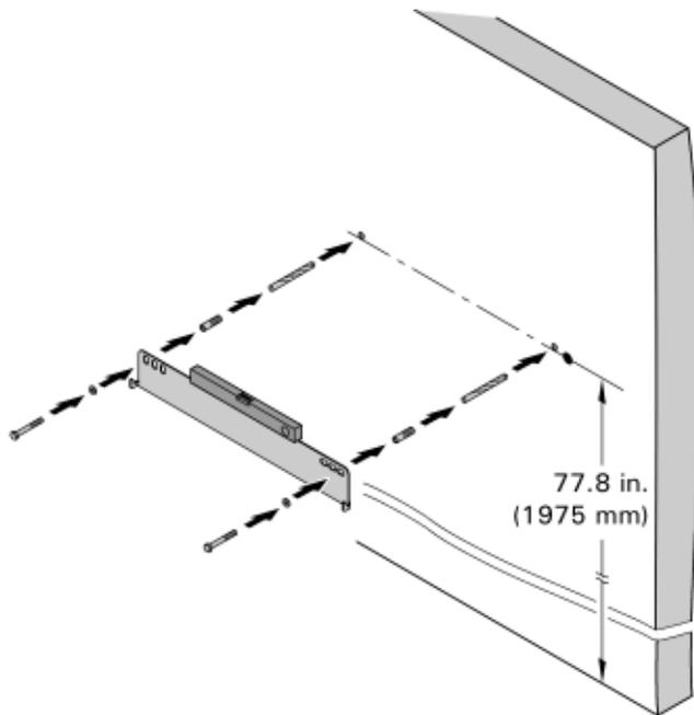
**Fitting the wall mounting bracket**
