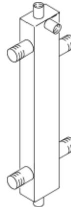
When used in conjunction with the Vitodens 200-W boiler, the low-loss header acts as hydraulic break, decoupling boiler and system circuits from each other. It is recommended to use the low-loss header in applications in which the total system flow rate exceeds the maximum (or minimum) boiler flow rate. For maximum boiler flow rates, starting on page 10 of this manual.
