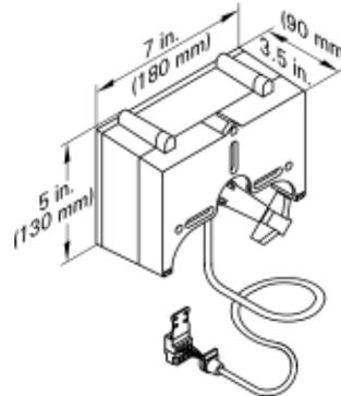
The mixing valve actuator is mounted directly on the Viessmann ¼ to 2½" mixing valve.
